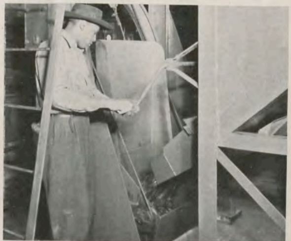
Fig. 2 — Filling the Wheelabrator Tumbblast loader from the storage hopper.
