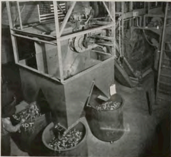
Fig. 6 — Four-way bin-dumping mechanism.
