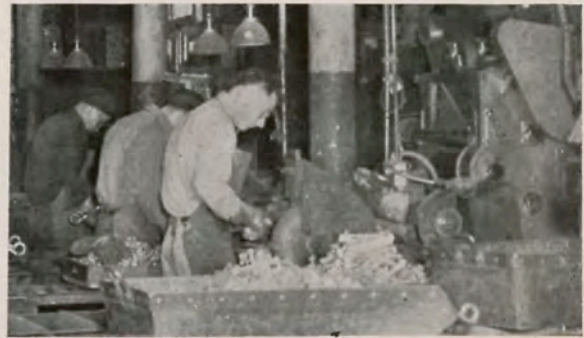
Fig. 3 — All brass castings are ground prior to Wheelabrating.
