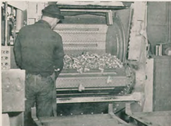
Fig. 1—Unloading brass valves from the 27" x 36" Wheelabrator Tumbblast.
