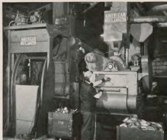
At the Syracuse Heat Treating Company, Syracuse, New York, one of the leading Eastern heat treating concerns, three Wheelabrator Tumblasts, a 15" x 20", a 20" x 27" and a 27" x 36", are employed to handle the complete cleaning of heat treated parts. With these machines they are equipped to process metal pieces weighing from a few ounces to over 75 pounds apiece.
