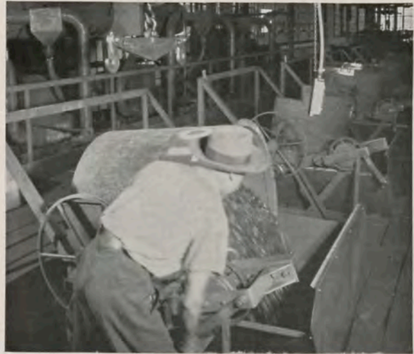
Fig. 1 — Dumping mechanism empties uncleaned belt links into storage hopper.
