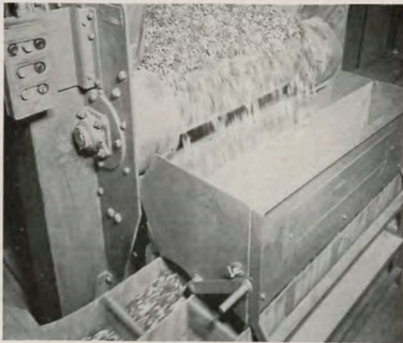
Fig. 5 — Closeup of unloading operations. Note split conveyor.
