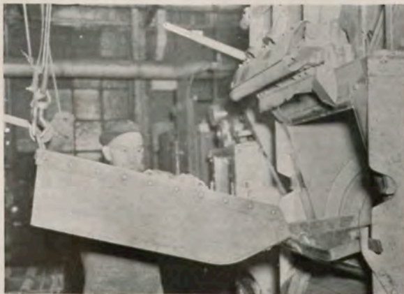
Fig. 4 — Loading the smaller Wheelabrator Tumblers is facilitated with this handling device.
